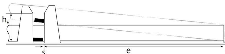
Figure 17.9 Height of transverse cover guides
